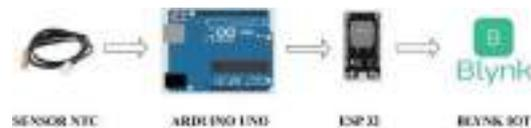
**Gambar 9** Proses transfer data nilai temperatur
