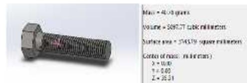
Gambar 51. Simulasi Solidwork Baut M10
