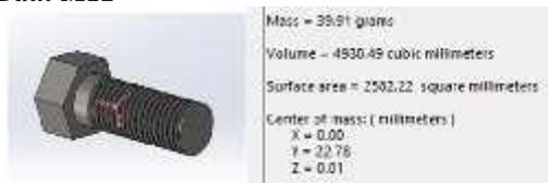
Gambar 55. Simulasi Solidwork Baut M12
